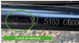
Outer Tie Rod installed with orientation arrow installed to rear of vehicle
