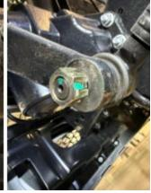
4. Use a ball joint separator tool to disengage the ball joints.
