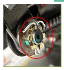
3. Remove the castle nut and turn it counterclockwise, the base should be aligned with the threads of the ball joint. Note: Please be careful not to damage the threads.
