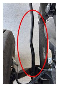
If tie rod orientation is rearward, proceed with the reinstallation procedure.
